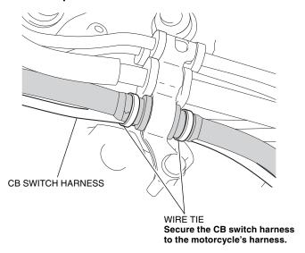
50. Secure the CB switch harness with the wire tie as shown.
