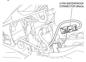
18. Remove the clip and disconnect the connector as shown.
