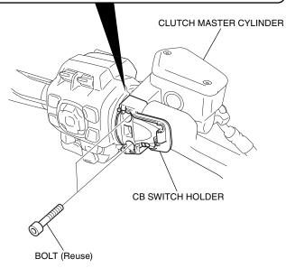
39. Install the CB switch case as shown.
